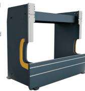
Press brakes feature a **rigid mono-block machine frame** for minimum deflection under load. The steel frame is checked by ultrasound and is stressrelieved after welding.
