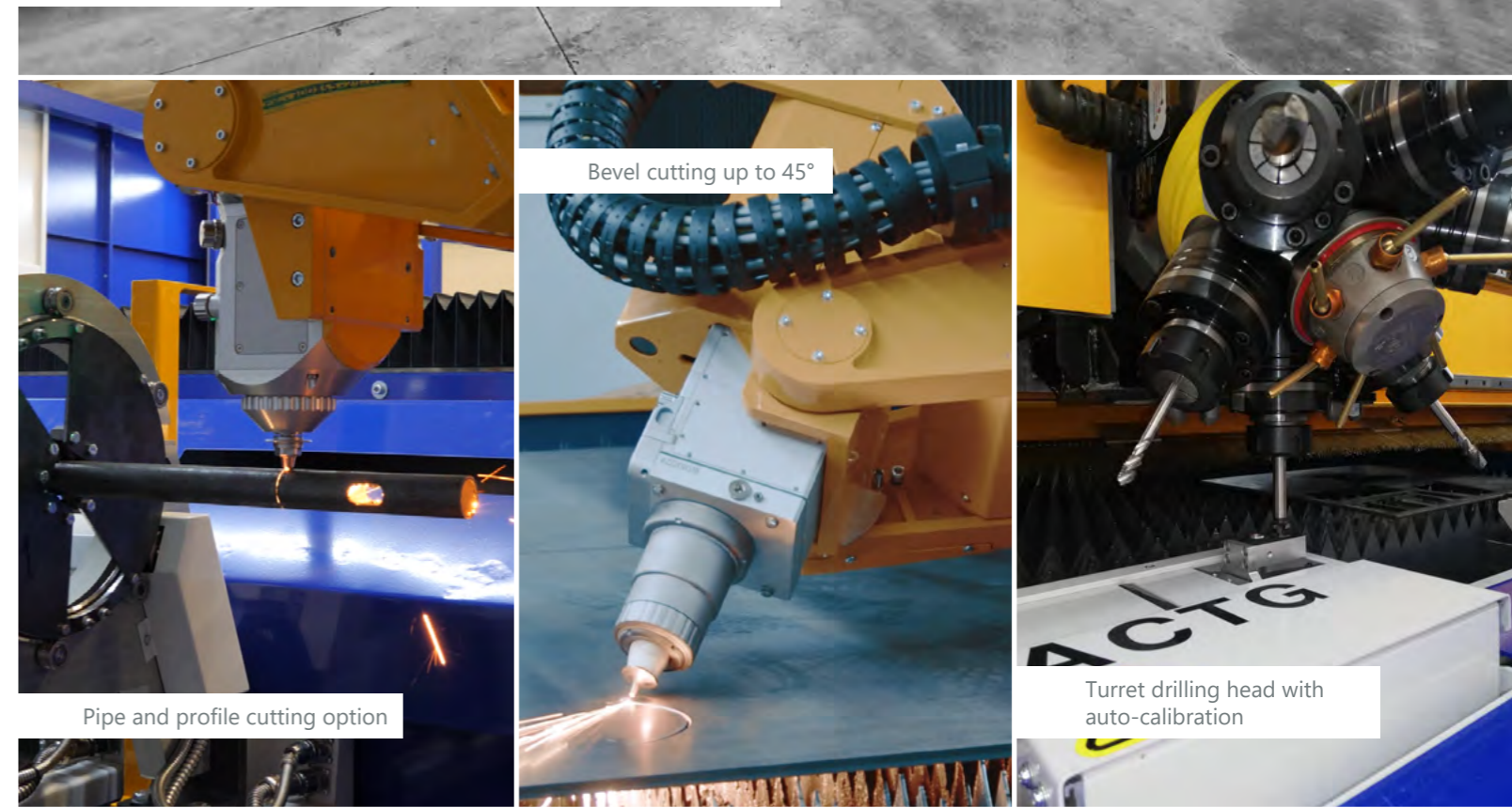
MSF Pro machines can be fully automated via material handling and sorting systems and CyberFab® Manager software
