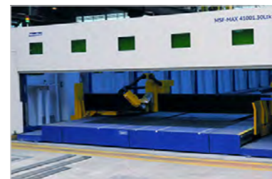
Laser bevel head for bevel cutting up to 45°
