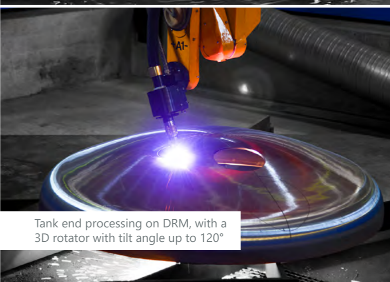
DRM machine with work area 50 x 8 meters and a water table for underwater plasma cutting
