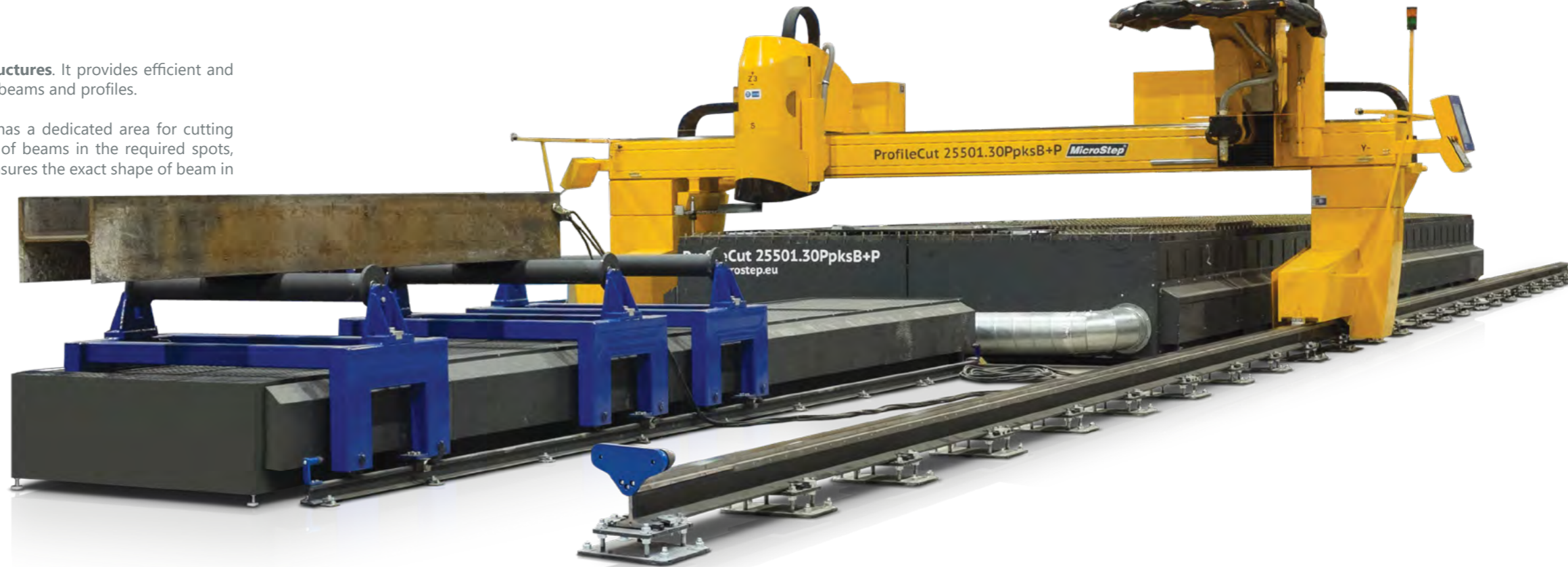
Great production flexibility thanks to the 120° bevel cutting head
