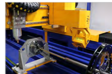
Laser scanner for measuring the true profile shape
