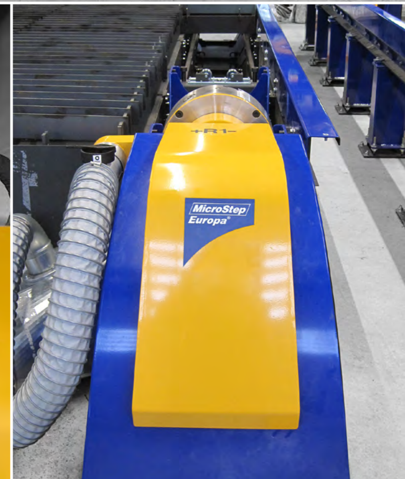
This pipe cutting device can process pipes up to Ø 300 mm
