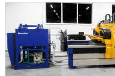
Abrasive removal system for cleaning of the water tank
