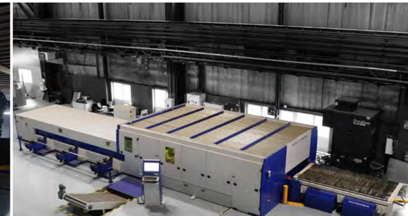
A combined machine with automated pipe cutting
