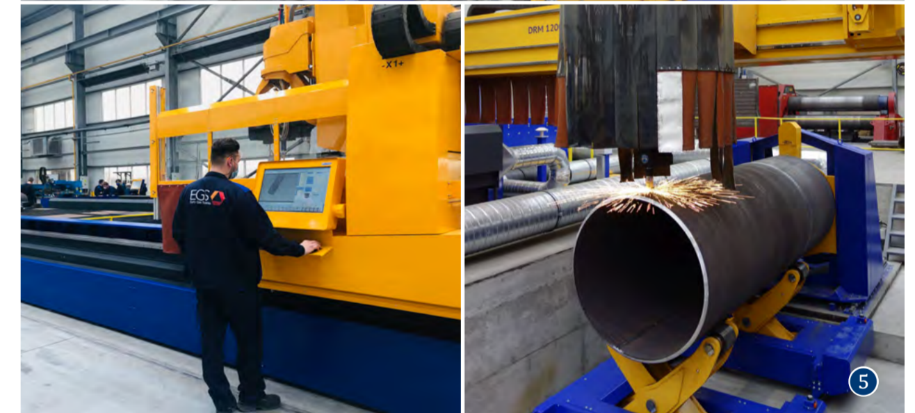
5 Plasma pipe cutting. The large positioner enables cutting of pipes up to Ø 2,000 mm, length 6 m and weight 7 tons.
