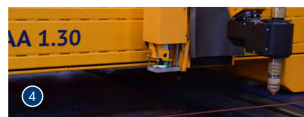
For the company Doppelmayr MicroStep installed a powerful drilling machine of the DRM series ① and two plasma and oxyfuel cutting machines of the MG series with two gantries ② + ③ each. The two MG machines are each equipped with a CCD camera ④ for maximum precision when cutting pre-drilled parts.
