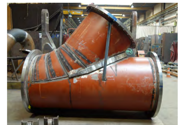
MicroStep delivered the complete cutting solution: with a 12 x 3 m large cutting area for plates up to 150 mm thick and a zone for cutting pipes with a robot situated along the outer side of the machine guides, the machine is capable of processing tubes up to Ø 2000 mm and wall thickness 80 mm.
