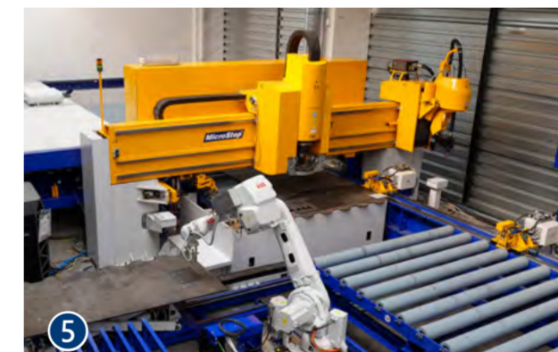
Plate processing line MicroStep DS with a 55 kW drill dedicated to automated production of flanges.
