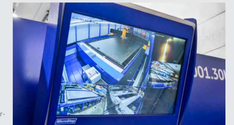
Simultaneous cutting, loading and unloading monitored from the operator console.
