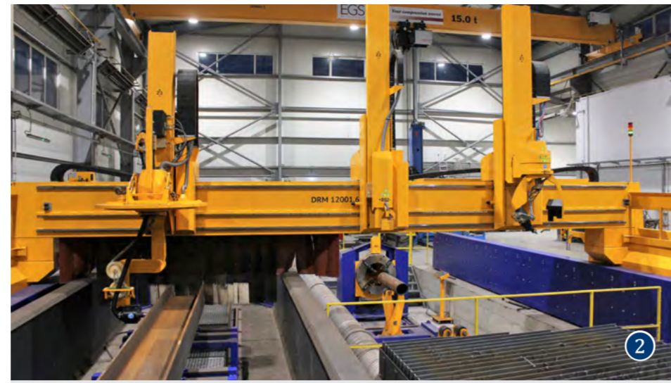
2 DRM gantry in EGS equipped with three tool stations. The machine has three work zones: cutting of beams (left), cutting of sheets and domes (front right) and cutting of pipes (rear right)
