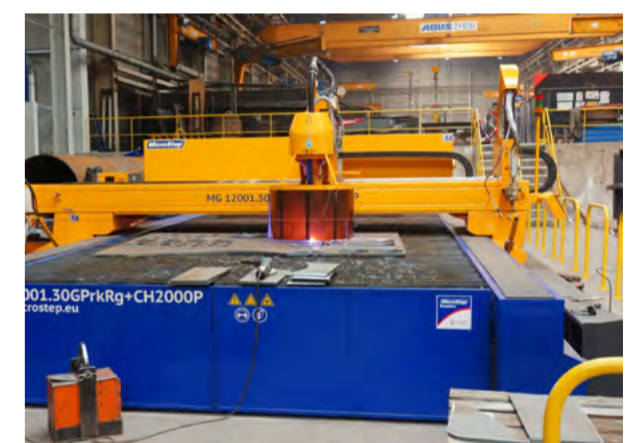
MicroStep delivered the complete cutting solution: with a 12 x 3 m large cutting area for plates up to 150 mm thick and a zone for cutting pipes with a robot situated along the outer side of the machine guides, the machine is capable of processing tubes up to Ø 2000 mm and wall thickness 80 mm.
