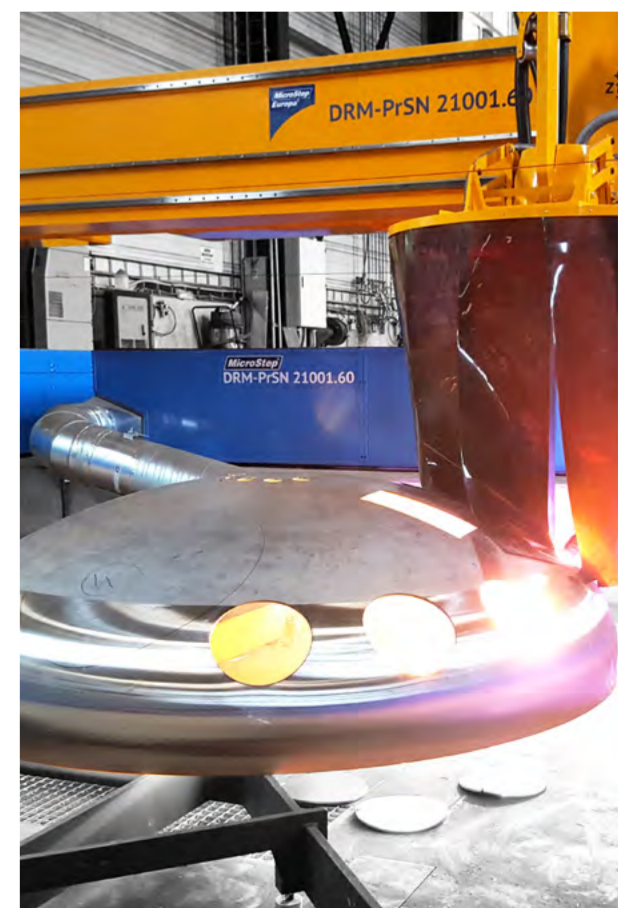
Maximum precision in dome cutting is made possible by MicroStep's mScan technology. In the process, a laser scanner integrated into the portal determines the 3D surface geometry of the workpiece in advance.
