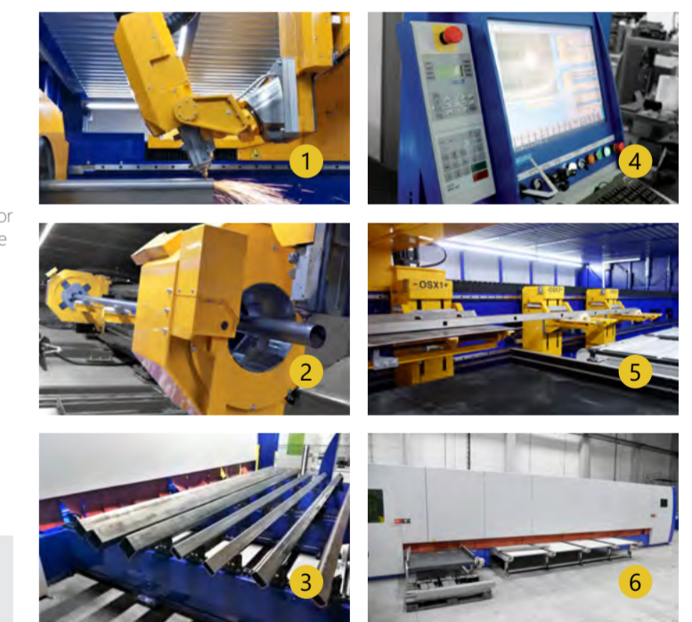
Automated pipe cutting machine MSF Pipe designed for 2D or 3D cutting of round pipes up to 6 m length and diameter Ø 200 mm as well as for tubes of rectangular and other cross-sections. The machine features a laser scanner that is used to determine the real shape of pipes to be cut to ensure accurate cutting results.
