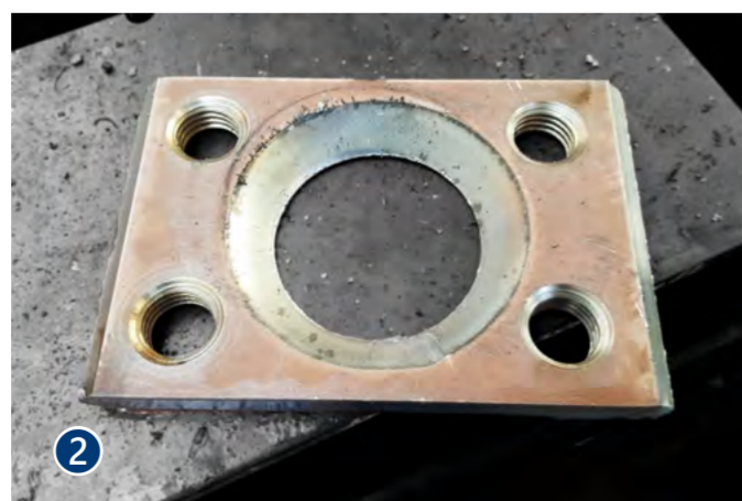
Hardox part drilled, tapped and bevel cut with plasma on a MicroStep DRM machine.
