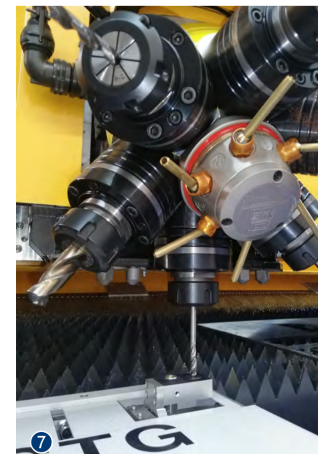
Calibrating a turret drill head on a MicroStep fiber laser machine with drilling/tapping/countersinking option.
