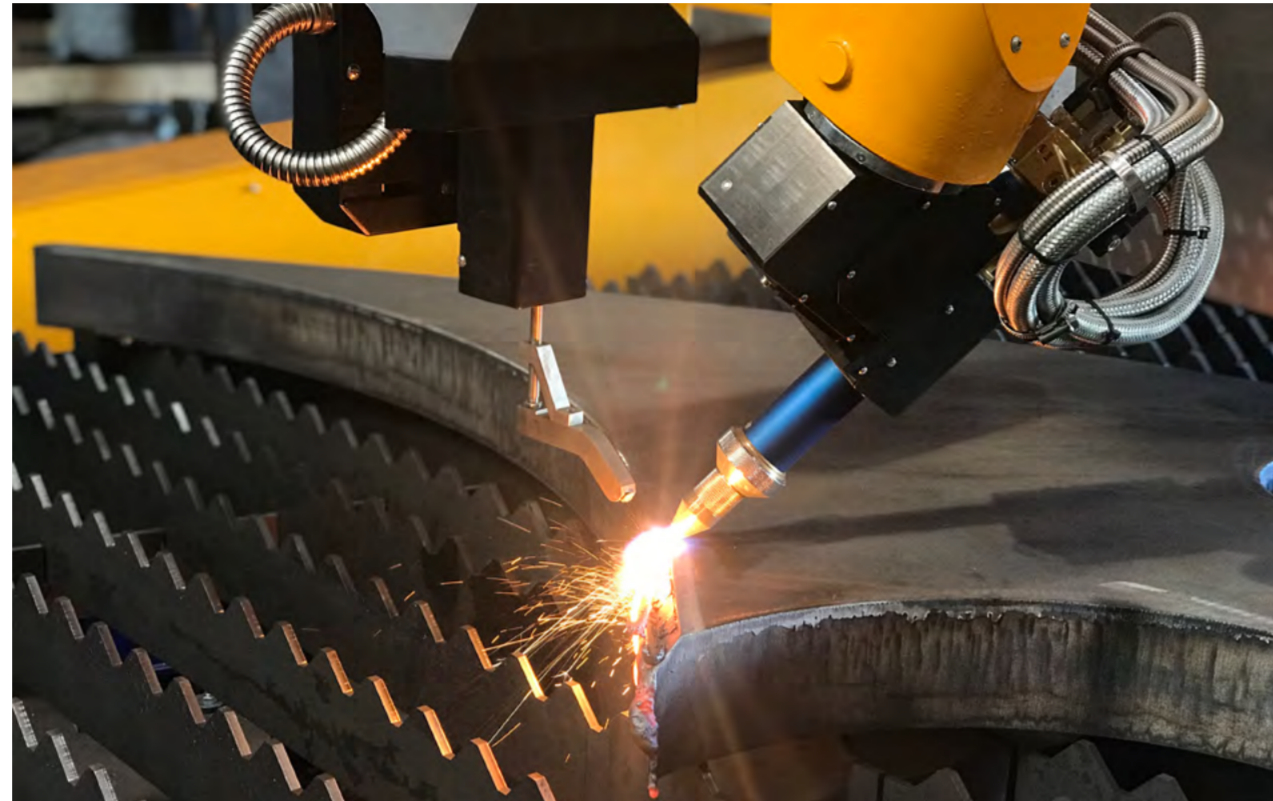
Oxyfuel rotator for weld preparation on thick metals utilizes MicroStep's patented ACTG® technology for automatic compensation of kinematic inaccuracies, and thus delivers reliable cutting results in the long run with a far less frequent maintenance necessary.
