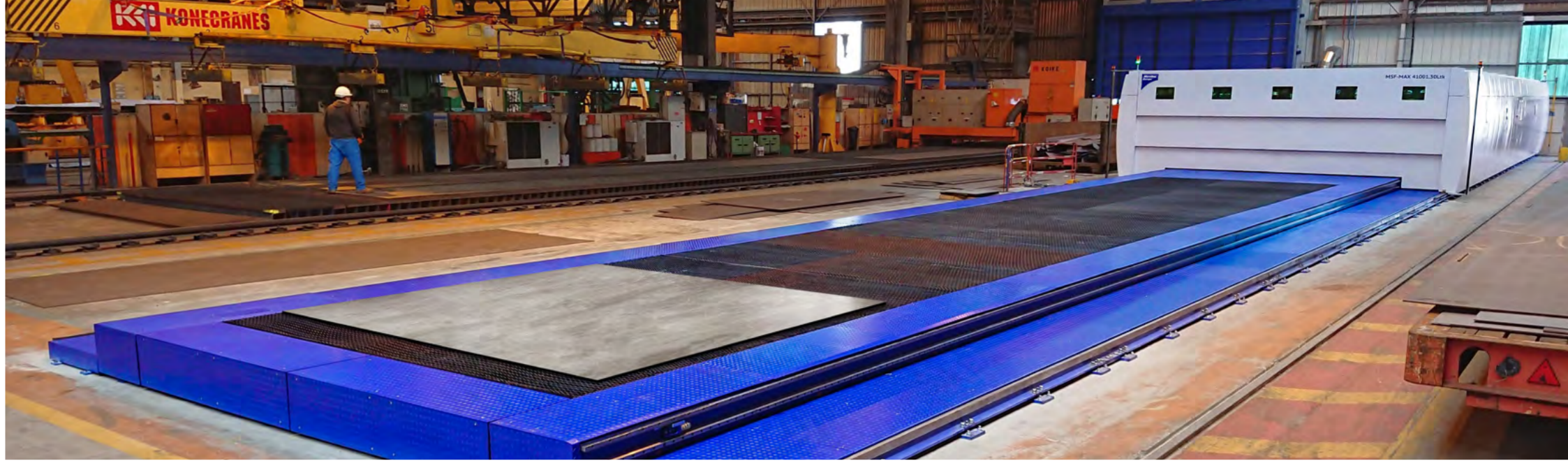
Above: Chantiers de l'Atlantique opted to invest into a large-scale fiber laser cutter MSF Max. It is a 50 m long machine with two 21,000 x 3,500 mm cutting zones.
