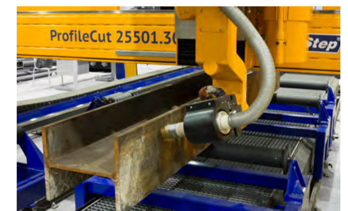
MicroStep has developed a variety of solutions for high-precision 3D processing of tubes, profiles and beams – including fully automated material handling.
