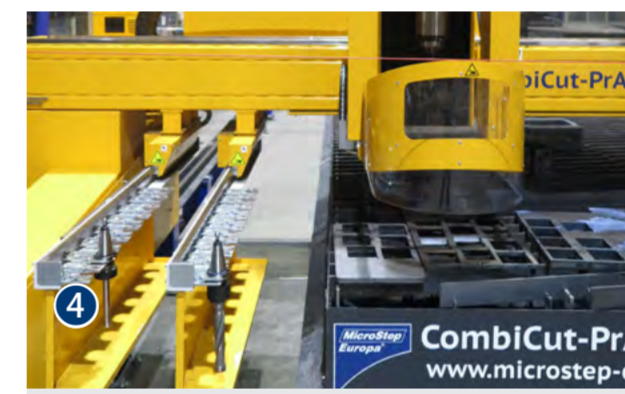
MicroStep drilling head with internal cooling and automatic tool change, with automatic tool magazines for 16 tools.
