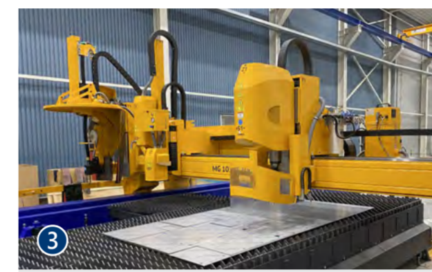
A multi-functional MicroStep machine with drilling up to Ø40 mm (+ tapping and countersinking), injet marking and a special plasma bevel head up to 120° tilt angle and endless rotation for plate, pipe beam and dome cutting.
